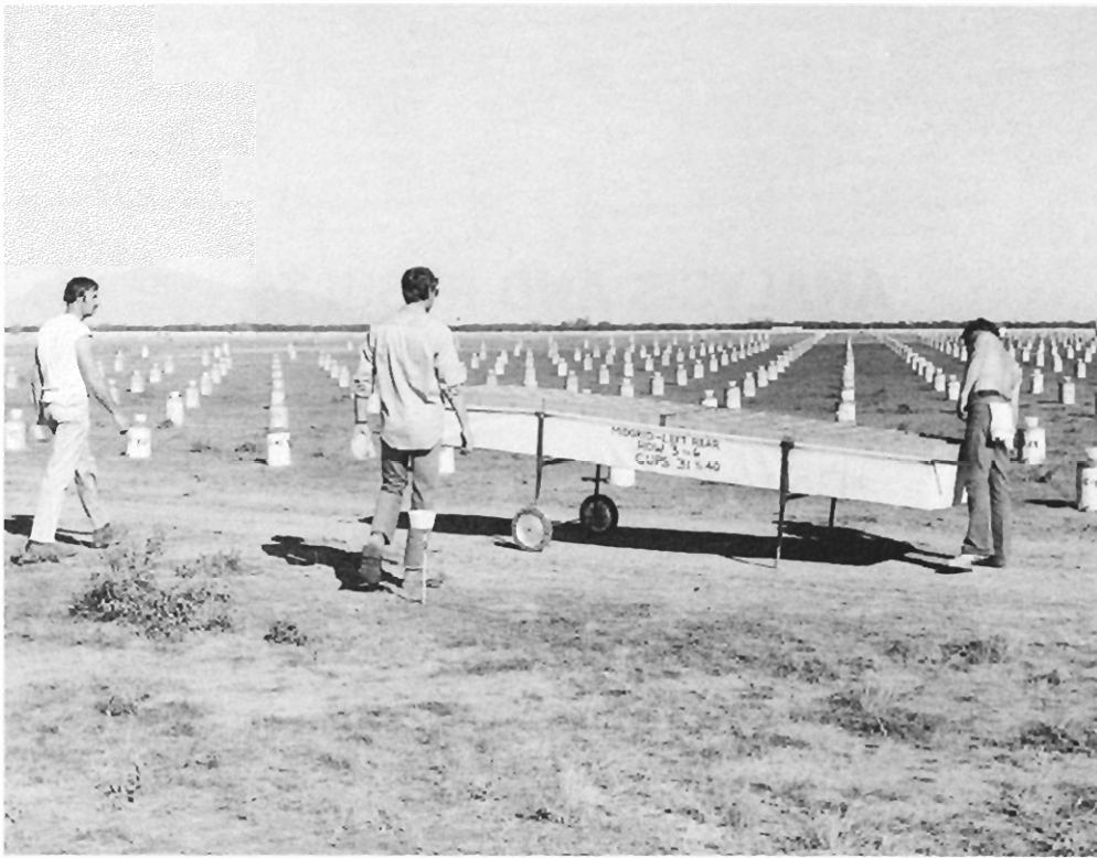
Figure 9.--Collecting the cups following several retardant drops.
